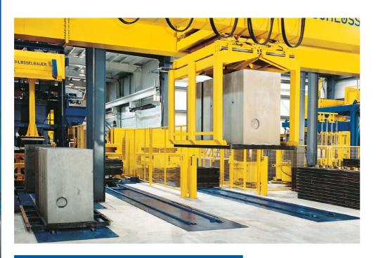
Production system for manhole components as well as reinforced and non-reinforced concrete pipe, road side channels, and pipe connection parts
