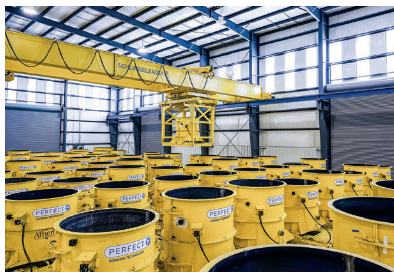
Transexact - Automated crane operation and mould management system in one.
