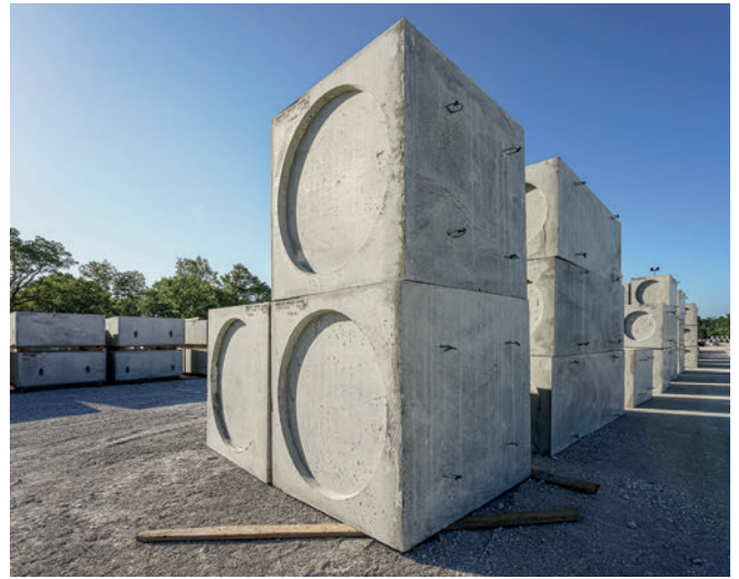
In addition to custom monolithic Perfect manhole bases, rectangular and standardized manhole components are also manufactured on the plant.
