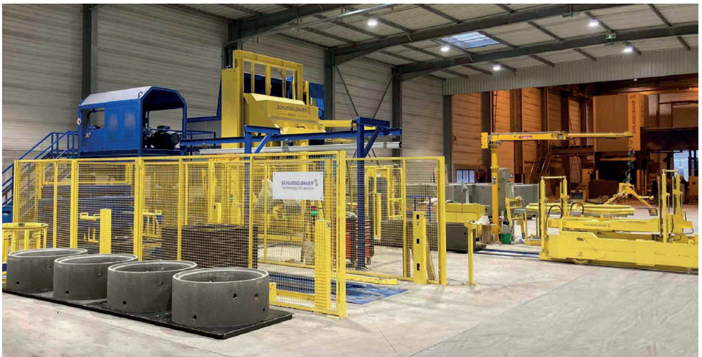
The new Magic 1501. Schlüsselbauer's Exact machine can be seen in the background.
