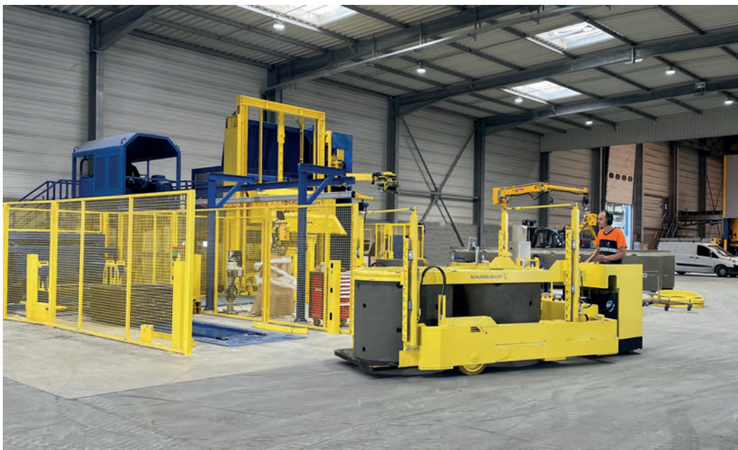
Anchors and step rungs are automatically positioned on the right of this photo, while the silo is offset behind the building wall. The Magic system was customized to fit the existing building.
