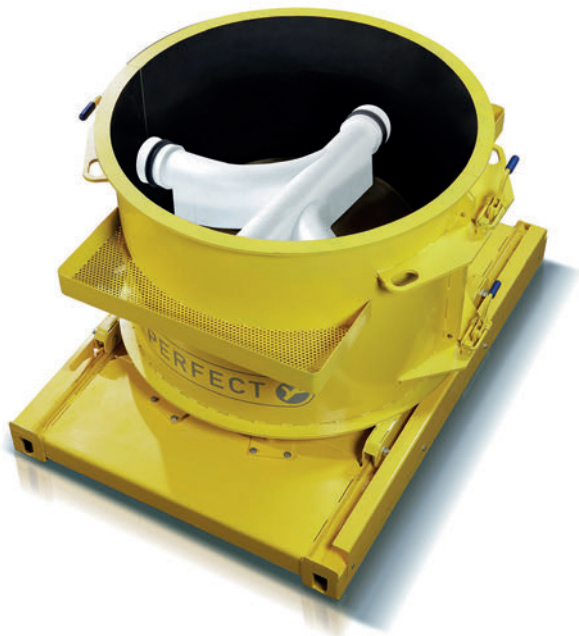
The completed channel with pipe connection parts is assembled in a casting mould. The mould is then ready for the SCC to be poured.
