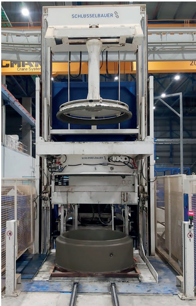
The Magic system for mass production of manhole risers with nominal widths of 800, 1000, 1250 and 1500 mm.
