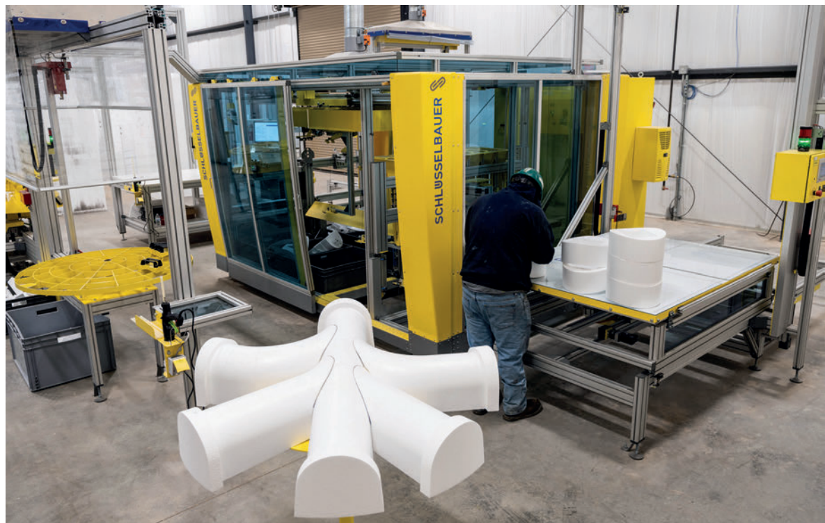
Production of a channel negative on the Perfect system; the image shows the complete channel with multiple pipe connections.
