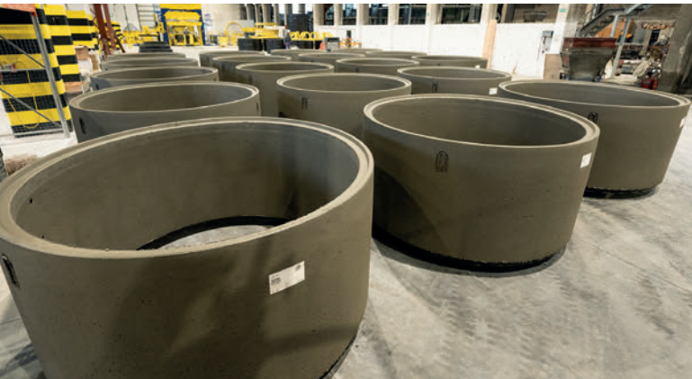
Up to 110 DN 2000 manhole rings or 90 DN 2500 manhole rings are manufactured in one-man operation at the Sollenau site every day.
