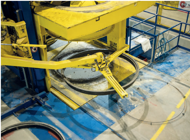
A steel bottom pallet is automatically transferred to the machine for each production cycle.
