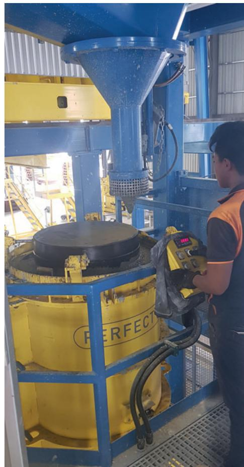
Filling the prepared moulds with self-compacting concrete
