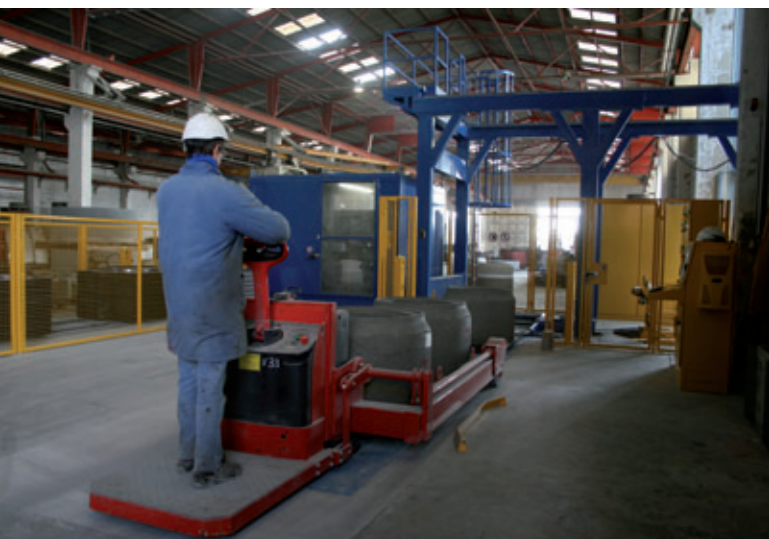
The hardened products from the previous day's production are moved to the loading station on the electric transport cart
